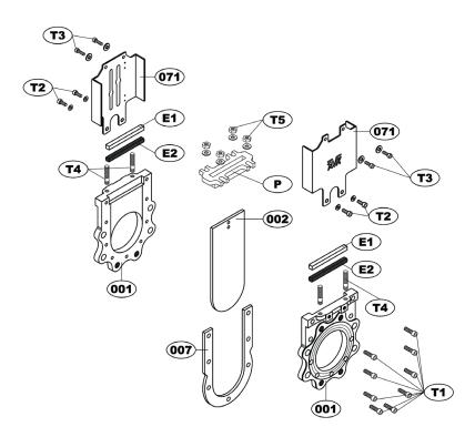
To change U-shaped sealing and packing gland material, proceed as follows:
