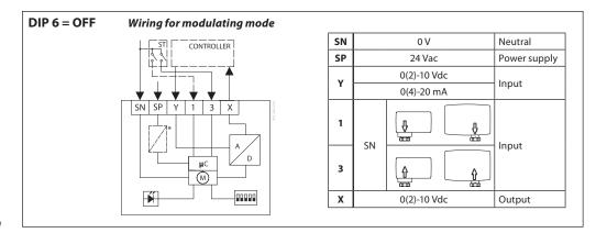
Actuator needs to perform Self-adjustment prior changing DIP 6 to ON. Output signal depends on DIP 2, 3&5 setting.
