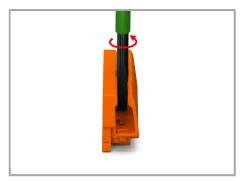
To adjust the mounting carrier, unlock the latch via operating tool (5.5 mm blade) and move the clamping slide to the required width by rotating the tool.
