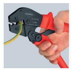
Third step: when greater hand force is required, such as e.g. when crimping insulated connectors  $6.0 \text{ mm}^2$ , two-hand operation is possible by the longer handles
