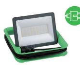
Model: IMT47226 Material : Aluminum+ABS Watt : 30W Voltage : 220-240V~50Hz Input current: 0.136A Lumen: 3000LM CCT: 4000K Size :225x231x40mm Net Weight : 980g Beam Angle : 110° PF : 0.9 Lighting area :0.028m<sup>2</sup>
