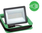
Model: IMT47228 Material : Aluminum+ABS Watt : 30W Voltage : 220-240V~50Hz Input current: 0.136A Lumen: 3000LM CCT: 4000K Size :225x231x40mm Net Weight : 980g Beam Angle : 110° PF : 0.9 Lighting area :0.028m<sup>2</sup> IMT47225 IMT47227
