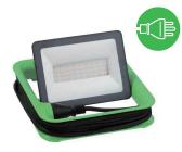
Model: IMT47227 Material : Aluminum+ABS Watt : 20W Voltage : 220-240V~50Hz Input current: 0.092A Lumen: 2000LM CCT: 4000K Size : 230x205x42mm Net Weight : 850g Beam Angle : 110° PF : 0.9 Lighting area :0.021 m<sup>2</sup>
