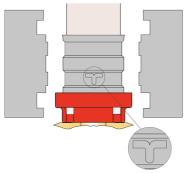
Logo illustration imprinted on the bush after pressing performed using a TH profile crimping tool—
