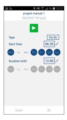
Enter the parameters (type, time, week day). The switching time can be entered either via the time picker or directly using the number pad.
