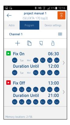
The copy, paste and delete functions (screens) are identical to the time switches.
