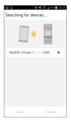
All the devices found appear in a list (devices with a Bluetooth dongle inserted). The device type and serial number (with the last four digits in bold) are displayed.
