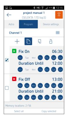
The selected switching times are now available on the clipboard and can be inserted again in any location (e.g. channel 2) via the "Paste" icon.
