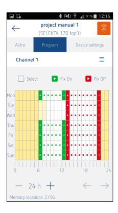
With graphical programming, you can touch the screen to set the switching times **for each channel** in a grid. The resolution (time unit per grid element) can be scaled using the zoom function "-24 h +" (1 hour, 30 minutes, 15 minutes). If the time unit is shorter than 1 hour (30 minutes, 15 minutes), you can scroll the programming area to the left or right with the arrows.
