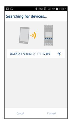
After selecting the required device, the connection is established and the project is transferred from the time switch to the app. Once data transfer is complete, a "Success" or "Error" message appears.
